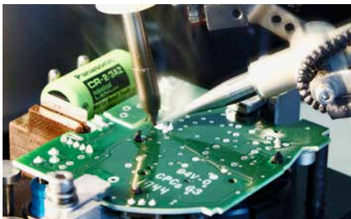
A soldering robot pictured at work on an Aico alarm
